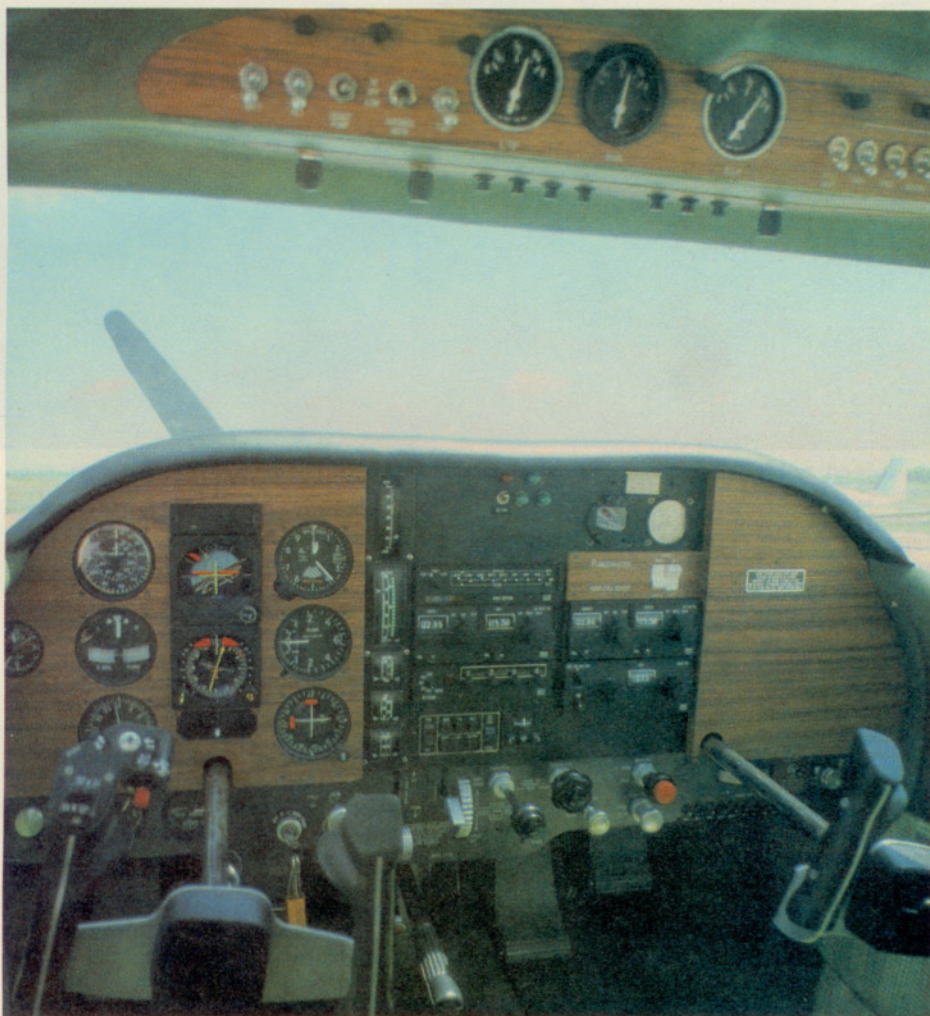
Note the unique location of controls above the Navion windshield and vertical readout engine instruments to the left of the radio stack.
