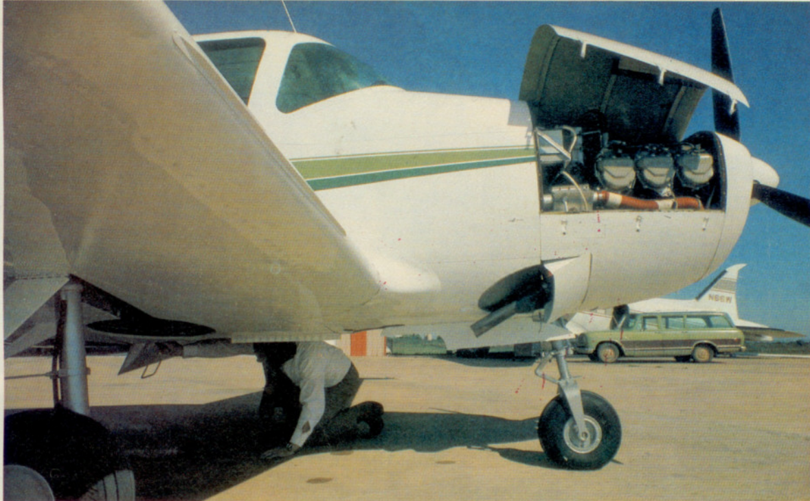
A pilot with Two Jacks, Inc. drains one of the three fuel sumps. Open cowl cover allows easy access to the engine compartment.
